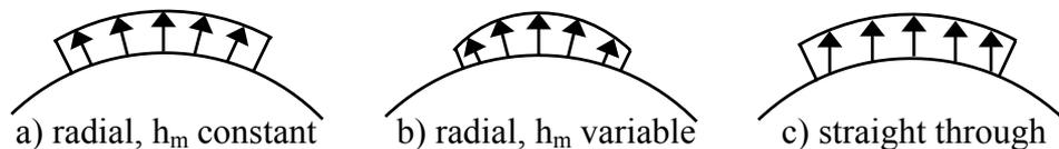
Figure D-1 Magnet shape and magnetisation
